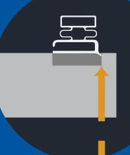
Measure from the outer edge of the seal for both the width and height of the seal.
