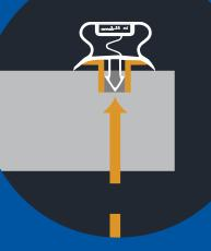
Measure from the center of the seal for both the width and height of the seal.
